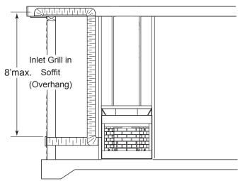
Figure 17 - Concrete Slab Installation (Optional Outside Air Runs)
